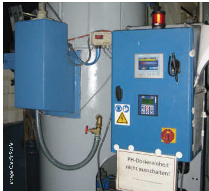
In conjunction with a specially developed additive, the dosing unit RDS-pH10 consistently maintains the pH value of the process water above a value of 10, preventing the formation of legionella.
