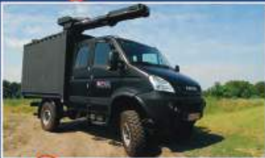
IFEX Firefighting System on IVECO Cross-Country Vehicle
