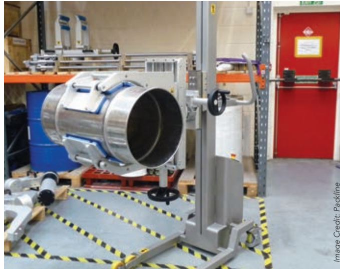
The new clamp attachment facilitates the positioning of rolls, drums and barrels
